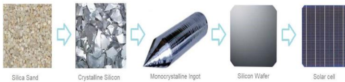
FIGURE 3: THE PROCESS OF TRANSFERRING SAND INTO A SOLAR CELL
