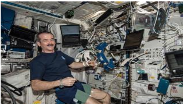
Figure(4): In support of the Blood Pressure Regulation Experiment (BP Reg), Chris Hadfield of the Canadian Space Agency is pictured after setting up the Human Research Facility (HRF) PFS (Pulmonary Function System) and the European Physiology Module (EPM) Cardiolab (CDL) Leg/Arm Cuff System (LACS) and conducting the first ever session of this experiment.
