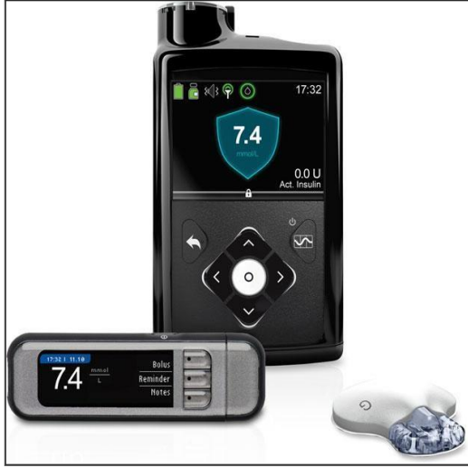
Figure 1: CLS is considered as one of the most promising devices for patients with Type 1 Diabetes, it consists of an insulin pump (the small cuboid-like apparatus) which may have the control algorithm inserted in it, a CGMS (the pieces at the bottom-right), and a communication device to enable doctors and experts to watch the device and patient state [11].
